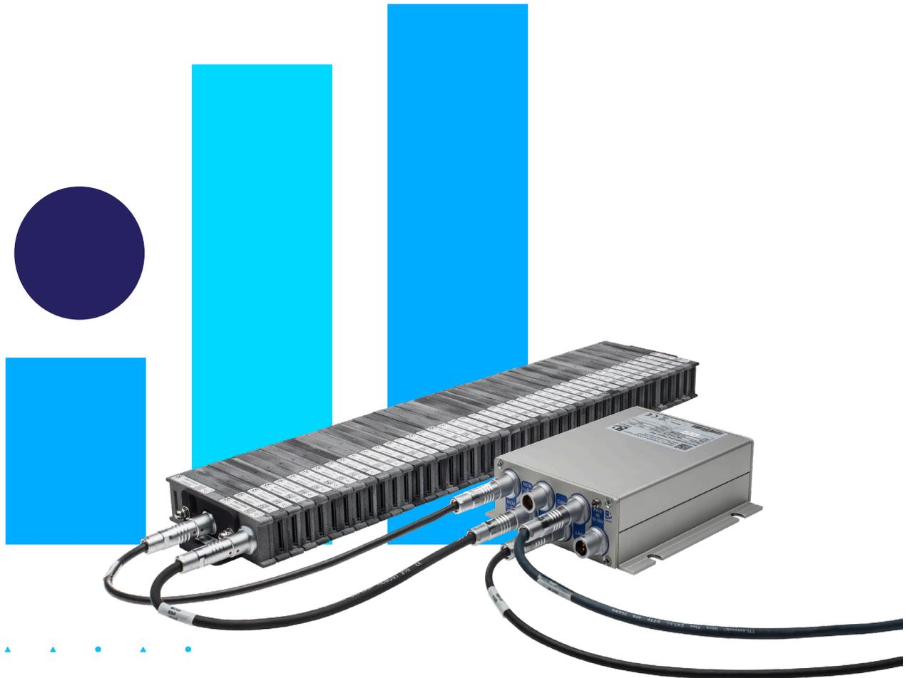
The Cell Voltage Monitoring (CVM) product family contains components for creating tailor-made cell voltage monitoring, simulation and processing systems. The decisive advantage of our modular concept is the great flexibility it offers for adaptation to cell stacks.
